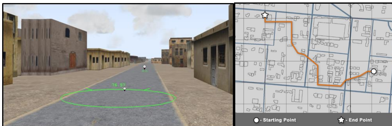
Figure 2: Sample imagery from the AR navigation simulation. Participants follow AR waypoints through a virtual city (left) while attempting to navigate a designated, safe pathway indicated on a map (right).
